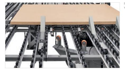
Front aligners to align the boards in the width directly on the turn station unit.
