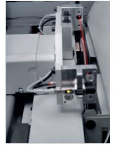
Automatic scoring blade alignment. The patented system automatically aligns the scoring blade in seconds. Supports the reduction of set-up times, test cutting and errors, increasing efficiency and reducing sharpening costs.
