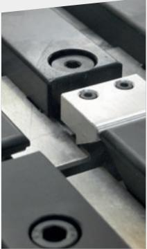
Cutting line closure system, to prevent the longitudinal trim cuts from falling into the machine and fouling the blade path.
