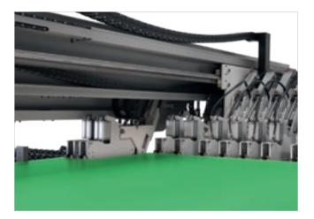
Device for simultaneous execution of staggered cross cuts, made with two completely separate pushers. Each pusher can choose to select two idle slave grippers (not powered) completely independently, based on the strips width to be cut. This unique solution allows to modulate the width of the two pushers and their working area.
