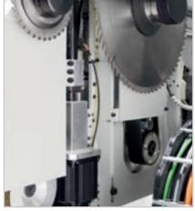
Motorised vertical movement of the blade ensures fast and **precise cutting height adjustment.**
