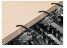
Panel clamping devices avoid the misalignment of the stack during the rotation phase
