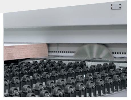
The double presser, with a double, independent structure, enables the application of consistent, controlled pressure to the stack of panels to be cut, thanks to the continuous gripper action, which also creates an actual sealed chamber for trim cuts and an efficient vacuum for the removal of dust.
