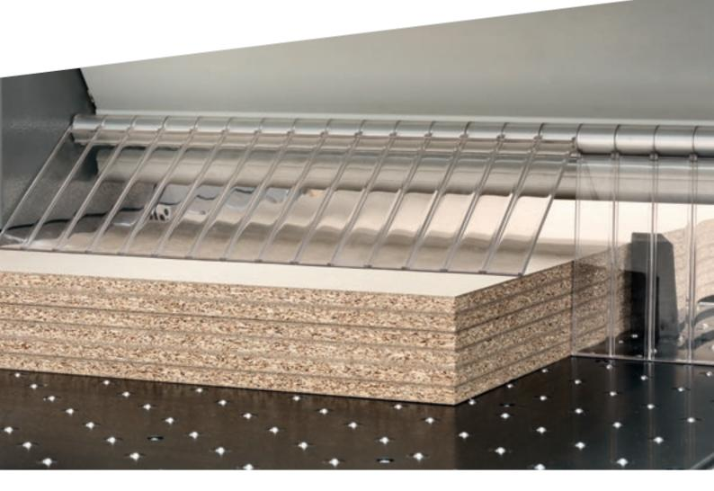
Side alignment stop integrated in the transversal blade carriage. Its features enable the perfect alignment of even the thinnest and/or most flexible panels, reducing cycle time to a minimum
