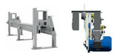
The optimal balancing and weight distribution on the two guides guarantees the total absence of vibrations and perfectly straight cutting action.
