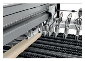
Device for simultaneous execution of staggered cross cuts, made with two completely separate pushers. Each pusher can choose to select one idle slave gripper (not powered) completely independently, based on the strips width to be cut.
