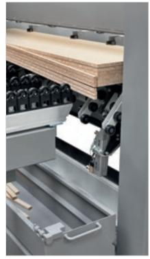
Longitudinal double-edge trims are disposed of by means of a dedicated and fully automated trapdoor with independent rollers.
