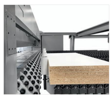
The stacks of strips are selectively transferred to the cross cut area according to the cutting cycle worked out by the Numeric Control.
