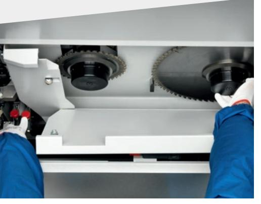
The "Quick change" system is the quickest, most ergonomic and safest device for changing blades without using tools.
